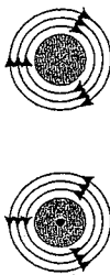
A dot in the center of the wire indicates electron flow out of the plane of the page, toward the reader. An "x" in the center of the wire indicates electron flow into the plane of the page, away from the reader.
